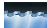
Tooth C coarse teeth with roughing tooth bevelled on both sides and finishing tooth not bevelled. The roughing tooth is about 0.2 mm higher
