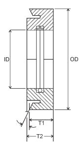
Bottom Shear Knives / Female Knives with Self-locking Type. (with Ball Bearing Balls)
